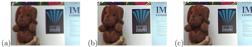
Figure 19: “Box Relaxation” - Example. A demonstration of the equation solution using “box relaxation” on the example of Sec. 5.1 (showing only a small part of the mid frame of the sequence). The boxes in this example were of size 7 \times 7[\text{pixels}] \times 79[\text{frames}] . (a) The initial state generated by an interpolation. Since the mid frame is far from the still images, the bi-linear interpolation is done only from the corresponding video frame (enlarging it by factor 3). (b) The solution after the first global iteration. Note the “blocky” texture over the image due to bad convergence of box boundaries. There are also trails of the moving toy that also did not converge well. (c) After 4 iterations the solution mostly converges.
