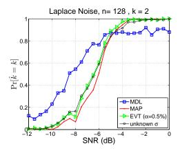
Fig. 5. Detection Performance with Laplace Noise.
