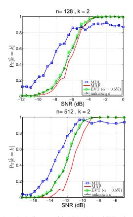
Fig. 3. Detection Performance of the MDL, MAP and EVT estimators as a function of SNR for record length n = 128 (left) and n = 512 (right) for the case of K = 2 sinusoids with closely spaced frequencies.
