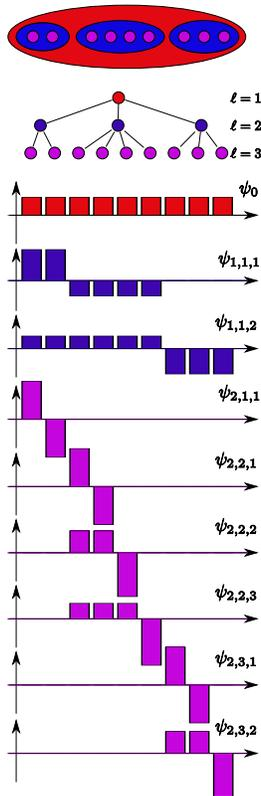
Figure 1. An illustration of a Haar-like basis.
