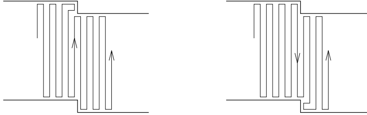
Figure 2.5: Deviation from columns scanning on strip steps
