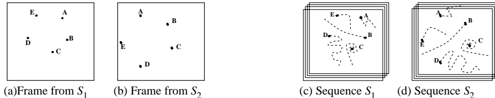
Figure 2: Point correspondences vs. trajectory correspondences. (a) and (b) display two frames out of two sequences recording five small moving objects (marked by A,B,C,D,E). (c) and (d) display the trajectories of these moving objects over time. When analyzing only single frames, it is difficult to determine the correct point correspondences across images. However, point trajectories have additional properties, which simplify the correspondence problem across two sequences (both in space and in time).
