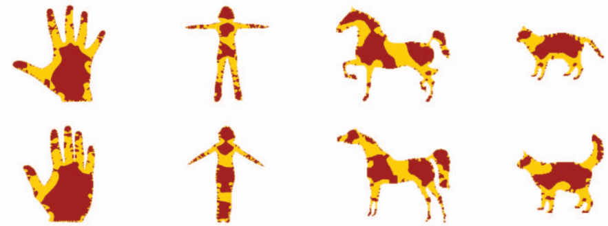
Fig. 13. A schematic representation of orientations computed via the Hessian matrix for several shapes. The turquoise color represents vertical regions ( |\alpha| \geq \frac{\pi}{4} ), yellow for horizontal ( |\alpha| < \frac{\pi}{4} ), and brown for isotropic sections \sqrt{|\lambda_{\min}/\lambda_{\max}|} \geq \frac{2}{3} . It can be seen that pairs of similar shapes give rise to similar orientation measures, but notice the thumb (left figure), which changes its orientation from near horizontal (top) to near vertical (bottom).
