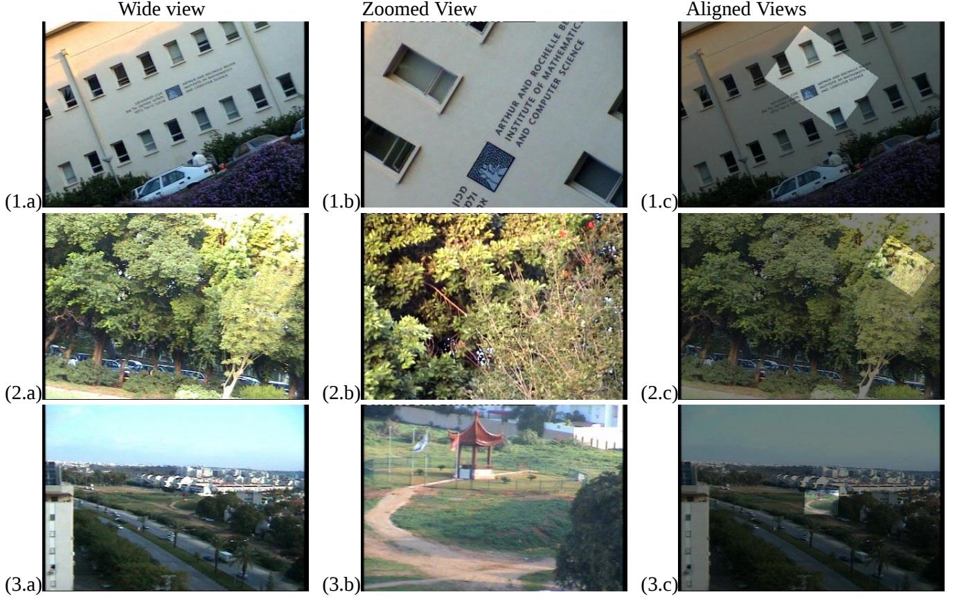
Figure 5: Finding zoomed region. This figure displays three different examples (one at each row), each one with different zoom factor. The left column (1.a, 2.a, 3.a) display one frame from each of the three wide-FOV sequences. The temporally corresponding frames from the corresponding narrow-FOV sequences are displayed in the center column (1.b, 2.b, 3.b). The correct time shift was automatically detected for each pair of narrow/wide FOV sequences. Each image on the right column shows super-position of corresponding frames of the two sequences after spatio-temporal alignment, displayed by color averaging (1.c, 2.c, 3.c). For full sequences see www.wisdom.weizmann.ac.il/NonOverlappingSeqs .
