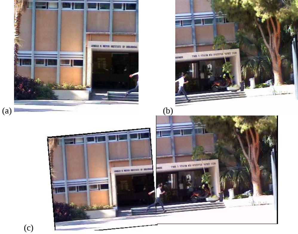
Figure 3: Alignment of non-overlapping sequences. (a) and (b) are temporally corresponding frames from sequences S and S' . The correct time shift was automatically detected. (c) shows one frame in the combined sequence after spatio-temporal alignment. Note the accuracy of the spatial and temporal alignment of the running person. For full sequences see www.wisdom.weizmann.ac.il/NonOverlappingSeqs .
