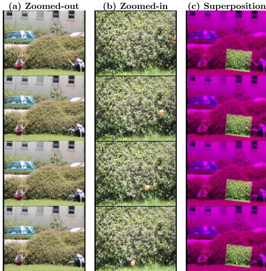
Figure 4. Alignment of sequences obtained at different zooms. Columns (a) and (b) display four representative frames from the reference sequence and second sequence, showing a ball thrown from side to side. The sequence in column (a) was captured by a wide field-of-view camera, while the sequence in column (b) was captured by a narrow field-of-view camera. The cameras were located next to each other (the spatial transformation was modeled by a homography) and the ratio in zooms was approximately 1 : 3. The two sequences capture features at significantly different spatial resolutions, which makes the problem of inter-camera image-to-image alignment very difficult. The dynamic information (the trajectory of the ball's center of gravity), on the other hand, forms a powerful cue for alignment both in time and in space. Column (c) displays superposition of corresponding frames after spatio-temporal alignment, using the algorithm of Section 3 for estimating the homography and the temporal correspondence between the two sequences. The dark (pink) boundaries in (c) correspond to scene regions observed only by the reference (zoomed-out) camera.
