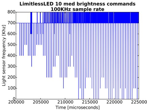
Figure 7. Decreasing brightness effect in high resolution
