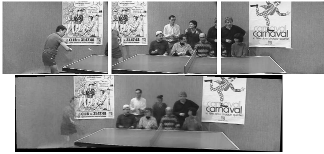
Figure 1: Static mosaic image of a table-tennis game sequence. Top row : Three out of a 300 frame sequence obtained by a camera panning across the scene. Bottom row : The static mosaic image constructed using a temporal median.
