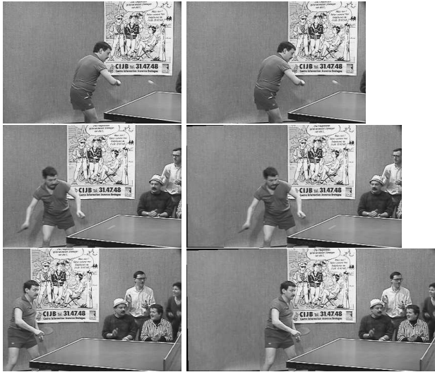
Figure 3: Evolution of the dynamic mosaic images of the table-tennis game sequence. Left column: Three frames from the original sequence. Right column: The corresponding dynamic mosaic images. Note that the position of the player and the crowd are constantly being updated to match the current frame.
