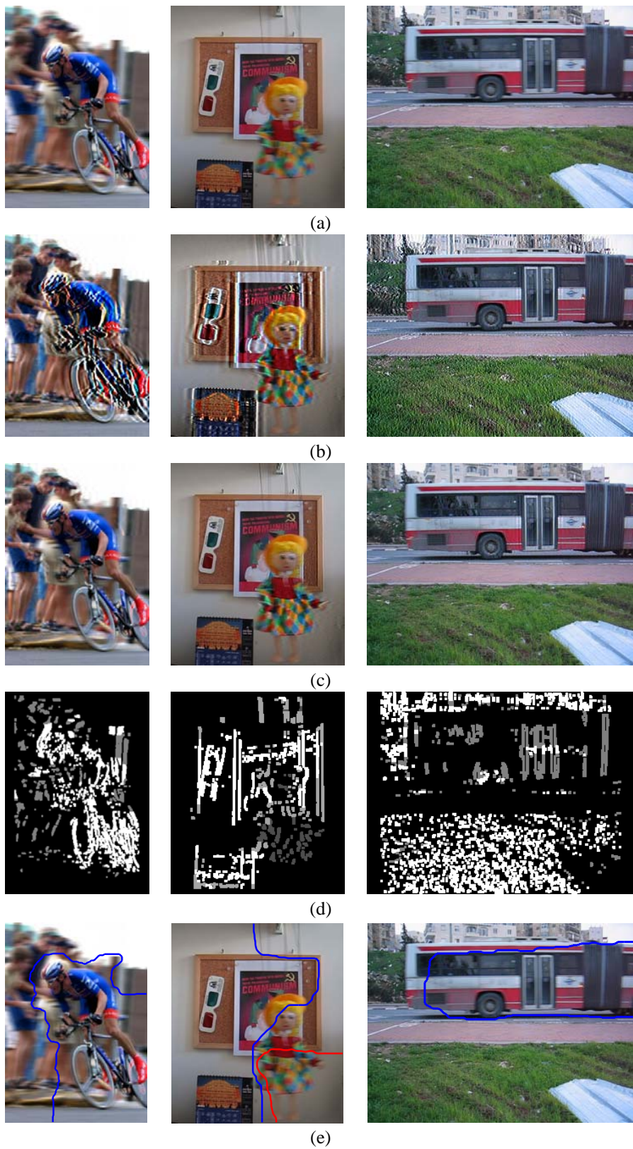
Figure 2: Deblurring Results. (a)Input image. (b)Applying the recovered kernel on the entire image. (c)Our result. (d)Local classification of windows. (e)Segmentation contour
