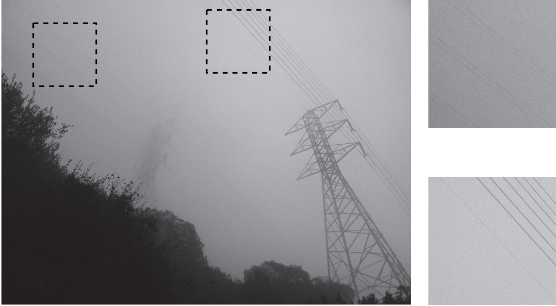
Figure 1. Power lines under poor visibility conditions. The extremely foggy weather leads to a low contrast and some barely visible edges. The image, of size 2592 \times 1936 pixels, contains two transmission towers, the left one barely visible. Some of the power lines are hardly visible, their existence inferred only by the presence of the transmission tower. On the right a closeup of two regions in the image—one with clearly visible power lines and the other with very faint ones.
