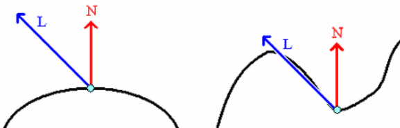
Figure 2: Two points with the same normal and light vectors have different illumination. The right one's light vector is blocked by the "hill" on the left of the plain causing it to be black.
