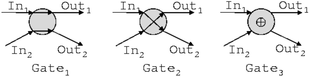
Figure 3: Some gates of a well-structured circuit. Gates 1–2 are switching gates, and gate 3 sits in layer 0 and computes the parity (xor) function.
