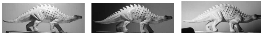
Fig. 5. Three out of 15 images with extremely near light (20 cm) used for photometric stereo reconstruction.
