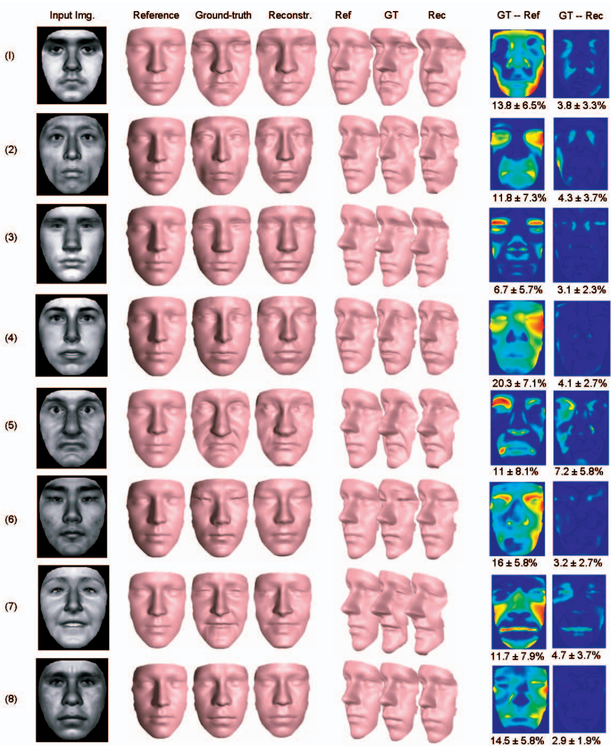
Fig. 3. Eight examples of typical reconstructions from the USF database. In each example, we show, from left to right, the input image, a triplet of shapes (the reference model, the ground truth, which is the laser scan, and our reconstruction) in two different viewpoints, and depth error maps ( 100 \cdot |z(x, y) - z_{GT}(x, y)| / z_{GT}(x, y) ) between the reference model and the ground truth (left) and between our reconstruction and ground truth (right). The colormap goes from dark blue to dark red (corresponding to an error between 0 and 40). The numbers under each of the error maps represent mean and standard deviation values in percents.
