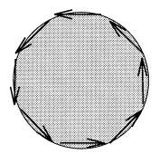
Figure 9. Discretizing a circle with a regular polygon.
