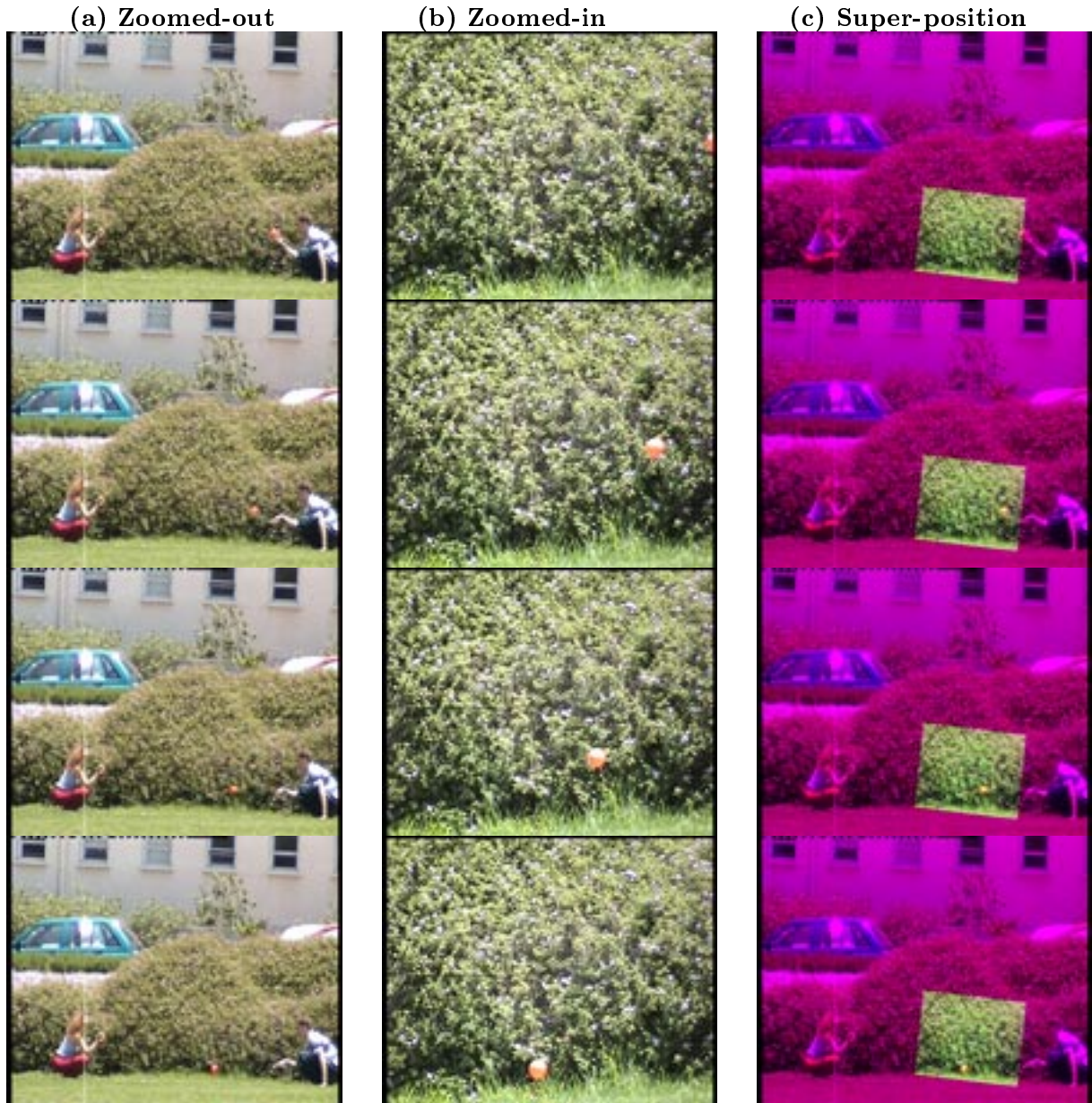
Figure 3: Alignment of sequences obtained at different zooms. Columns (a) and (b) display four representative frames from the reference sequence and second sequence, showing a ball thrown from side to side. The sequence in column (a) was captured by a wide field-of-view camera, while the sequence in column (b) was captured by a narrow field-of-view camera. The cameras were located next to each other and the ratio in zooms was approximately 1 : 3. The two sequences capture features at significantly different spatial resolutions, which makes the problem of inter-camera image-to-image alignment very difficult. The dynamic information (the ball's center of gravity trajectory), on the other hand, forms a powerful cue for alignment both in time and in space. Column (c) displays superposition of corresponding frames after spatio-temporal alignment, using the algorithm of Section 3 for estimating the homography and the temporal correspondence between the two sequences. The dark pink boundaries in (c) correspond to scene regions observed only by the reference (zoomed-out) camera.
