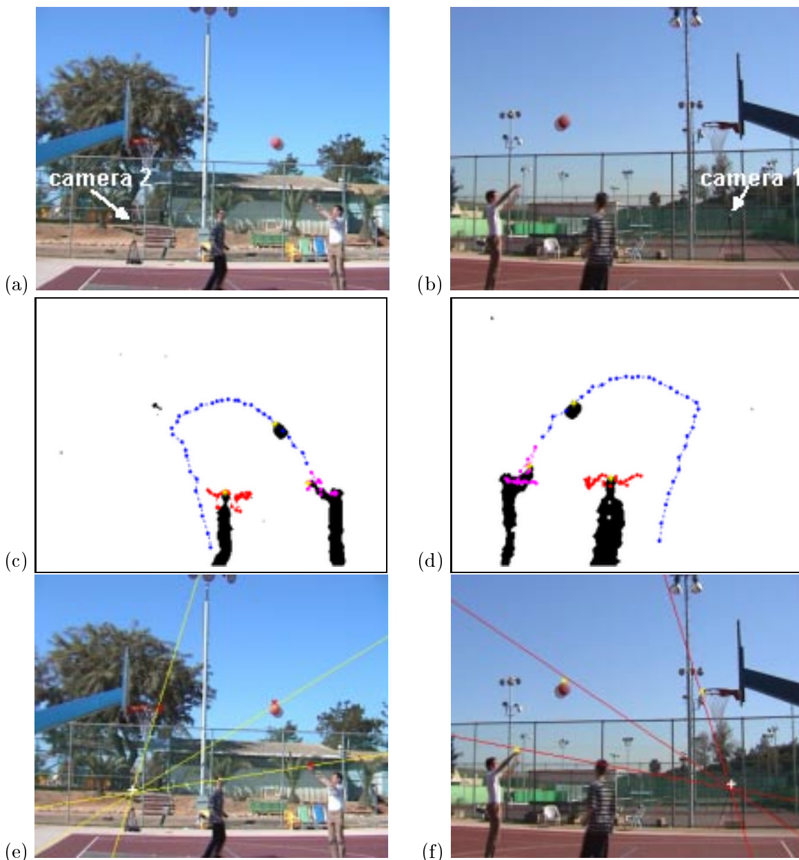
Figure 6: Wide Base-Line Matching (a) and (b) display two representative frames from two sequences of a basketball game taken from two opposite sides of the basket field. Each camera is visible by the other camera and is marked by a white arrow. Space-time trajectories induced by moving objects (ball and players) are displayed in (c)-(d) in different colors for the different objects. The tracked feature points that correspond to the current frame are marked in yellow. The recovered epipolar geometry is displayed in (e) and (f). Points and their epipolar lines are displayed in each image for verification. Note, that the only static objects that are visible in both views are the basket ring and the board. Accuracy of the recovered spatial alignment can be appreciated by distance of a point to the epipolar line of its corresponding point, as well as by comparing the intersection of epipolar lines with the ground truth epipole marked by a cross (the other camera).
