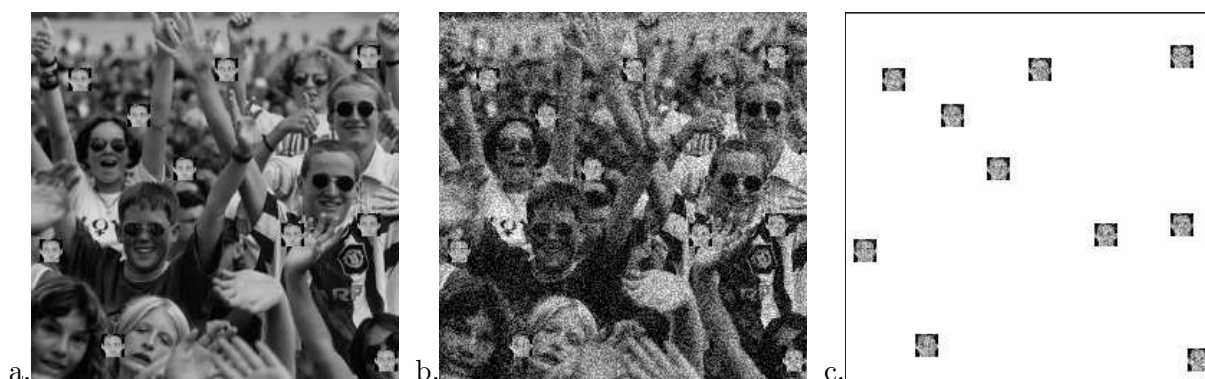
Figure 13: a. Original 256 \times 256 image containing several repeated patterns of size 16 \times 16 positioned randomly in the image. b. Very noisy version of original with noise level set to 40 (see text). c. All noisy patterns were detected.
