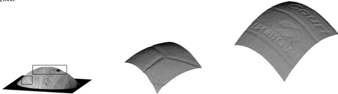
Figure 2. Blowups of the reconstructed volleyball (using the 4D method) reveals the stripes (middle) and the logo and writing (right).
