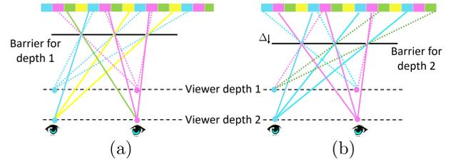
**Figure 3:** The depth sensitivity of parallax barriers: (a) A viewer at depth 1 sees at each eye rays from the same angular image. However, this no longer holds when the viewer distance is changed, as rays from different angular images converge at the same viewpoint. (b) Changing the distance between the barrier and the screen can adjust the display to a different viewer distance, but no barrier position can accommodate all viewing distances simultaneously.
