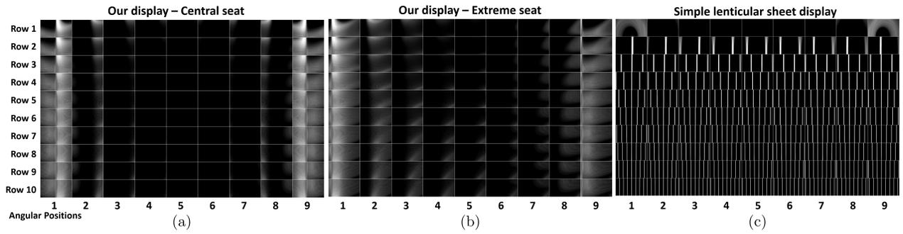
**Figure 12:** Transition maps of images viewed from our display, from the central seat (a) and the leftmost seat (b), in all cinema rows, relative to transition maps viewed from a simple lenticular sheet display, from a central seat (c). The maps are similar at the extreme seats. In the first row the viewed images are free of artifacts (besides the extreme angular positions 1 and k); however, when a viewer changes his distance, strong transition artifacts appear.
