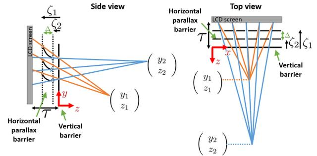
**Figure 4:** Display principle: For each viewer  $(y_i, z_i)$  (orange and blue), there exists  $\zeta_i$  such that a barrier placed at that screen distance leads to proper disparities for viewers at distance  $z_i$ . Concatenating all row-dependent barrier positions  $\zeta_i, i = \{1, \dots, m\}$  provides the desired shape of the slanted horizontal parallax barrier.
