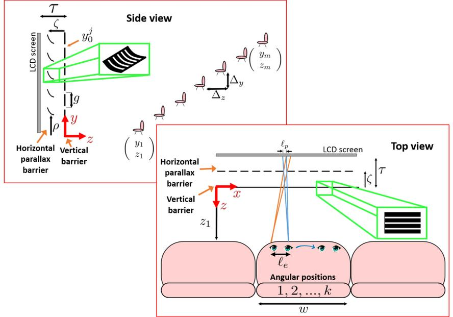
number of rows in the displayed images. The horizontal parallax barrier is located behind the vertical one. This horizontal barrier is a set of slanted surfaces with  $n_x$  vertical slits, whose structure is derived below.
