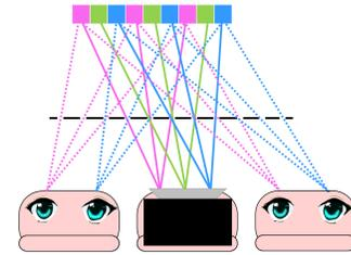
**Figure 17:** Our display can be used with a passive reflective diffused screen if we replace a single seat in a row with a multi-view projector. The projected multi-view content propagates to the passive screen via the display barriers. Due to the diffused nature of the screen, it spreads back toward all other seats in the row.
