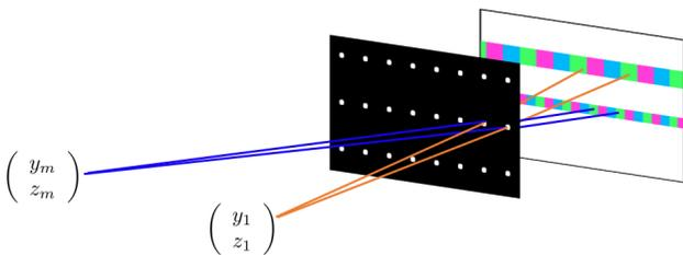
**Figure 10:** A naive automultiscopic display, composed of a pinhole array and a screen where each viewer row sees different pixel rows on the screen. To enable coherent content, one needs to use different horizontal scaling on the angular images intended for viewers in different rows. Thus, resolution tradeoffs here are worse compared to our design.
