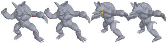
Figure 4: Deformations of the Armadillo using Mean Value Coordinates, and their bounded-distortion approximation. Flipped and highly-distorted ( > 25 ) tets are highlighted.
