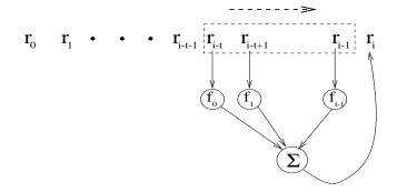
Figure 8.5: The LFSR small-bias generator (for t = k/2).
