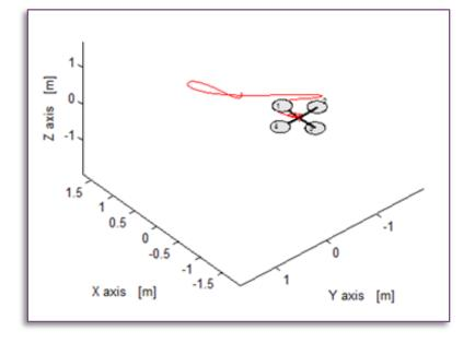
Results of applying the quadrotor Simulink model of Bouabdalla et al where a linear transformation box is replaced with behavior threads.
