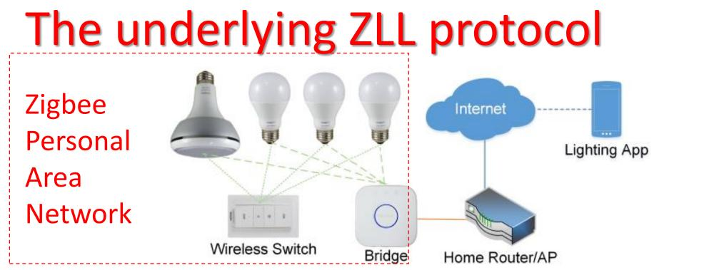
• Each installed light is connected to a central controller using the ZigBee Light Link (ZLL) wireless protocol in a Personal Area Network (PAN)
