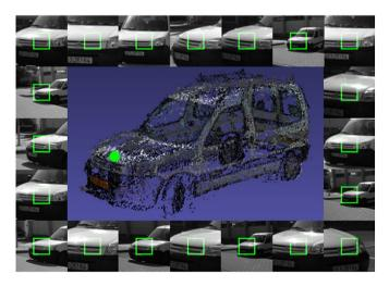
**Fig. 1.** 2D appearances: An example of the different 2D appearances  $\{e\}$  of a 3D point **I** (denoted as a green dot) as seen from different view-points and scales (corresponding to different training image indices *t*).
