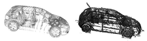
Fig. 5. Comparing CAD and SfM. We compare a CAD model (left) to the point cloud reconstructed using [2] and [3]. Using ICP we align the two models and measure the errors. The median error is 1.6 cm, less than one percent of the car's width.
