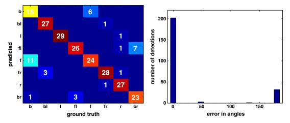
Fig. 7. Stanford 3Dpose cars - pose estimation. A confusion matrix and a histogram of label differences. Average accuracy is 85.28%.
