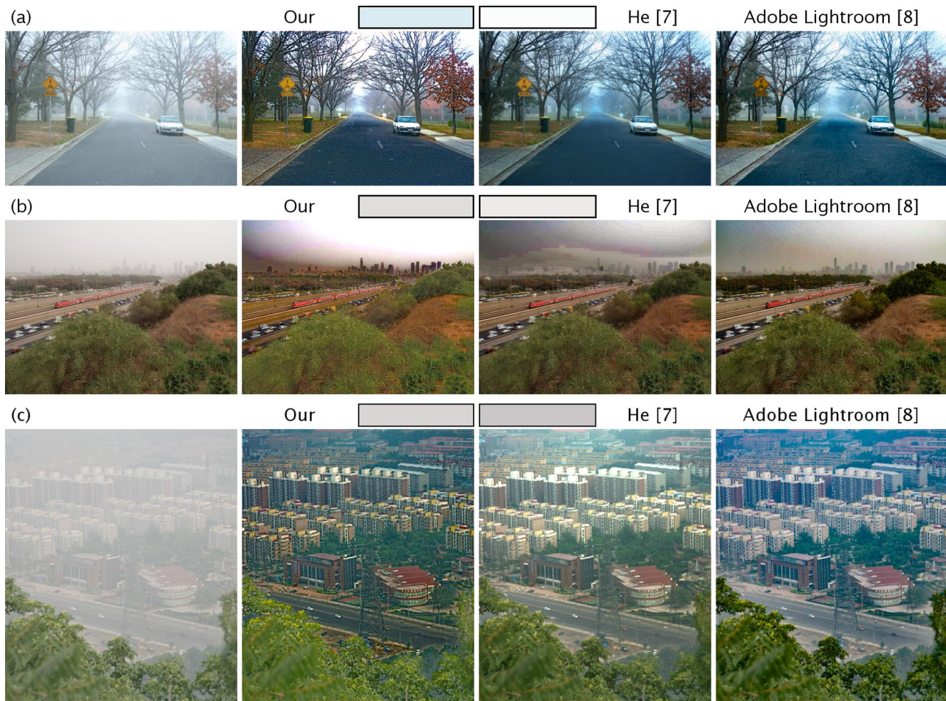
Figure 5. Dehazing results on images containing heavily-hazed distant scene points: The hazy input image (first column), our blind dehazing result (second column), result by [7] (third column) and the results using [8] (last column). The recovered airlight color \hat{A} of our and He’s dehazing results is presented in a framed rectangle above it. (Best viewed on screen.)
