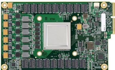
Can be inserted into a SATA hard disk slot for easy/fast deployment to existing server infrastructure
