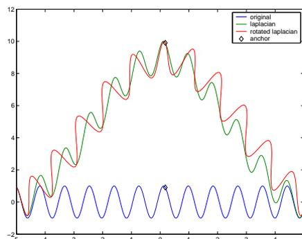
Fig. 1. The differential coordinates are not rotation-invariant. Therefore, when we edit the mesh (lower curve), the orientation of the details with respect to the low-frequency surface is not preserved. To rectify this, we explicitly rotate the differential coordinates (see the dark curve).
