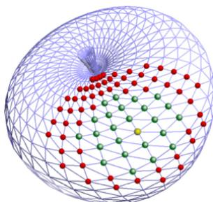
Fig. 2. Classification of the vertices of the edited region (ROI). The yellow vertex is the handle vertex which is moved by the user. The green vertices are the *free* vertices of the ROI (their position changes according to the reconstruction process). The red vertices are the stationary anchors - their position is constrained in the least-squares sense.
