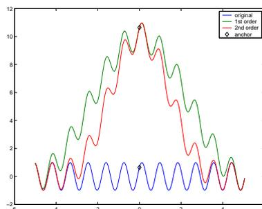
Fig. 3. The effect of editing the mesh (in blue) using different orders of the Laplacian operator. The constrained anchors are the left- and rightmost vertices of the mesh. Pulling the handle vertex in the middle results in the green curve for the 1st-order Laplacian and red curve for the 2nd-order Laplacian operator.
