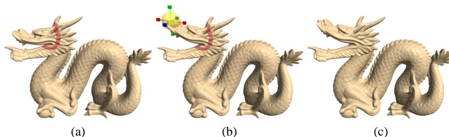
Fig. 5. Example of editing results using implicit optimization of local transformations. (a) The user selects the region of interest – the upper lip of the dragon, bounded by the belt of stationary anchors (in red). (b) The chosen handle (enclosed by the yellow sphere) is manipulated by the user: translated and rotated. (c) The editing result.
